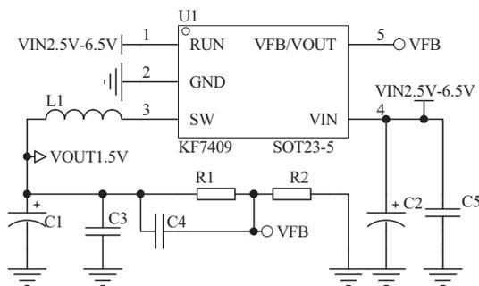
Figure 1. Basic Application Circuit with KF7409 adjustable version
